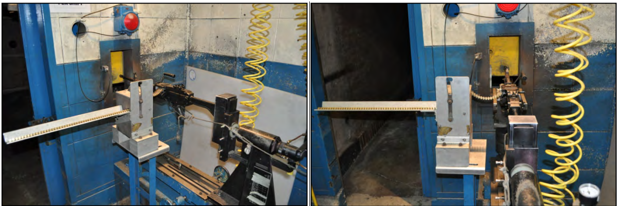
Figure. 6-B-6: Two views of the 5.56mm NATO Chute portion of the Function and Casualty Test with the MINIMI Mk1 Machine Gun
