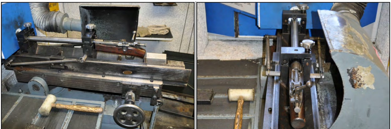
Figure. 6-B-9: Two views of the set-up for the 7.62mm Precision Test
