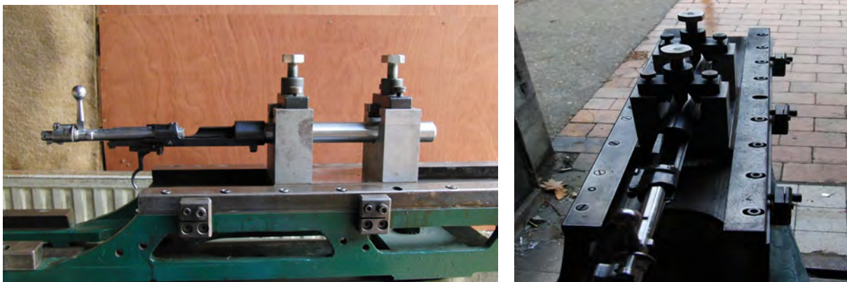
Figure. 6-B-8a: Two views of the set-up for the 5.7mm Precision Test
