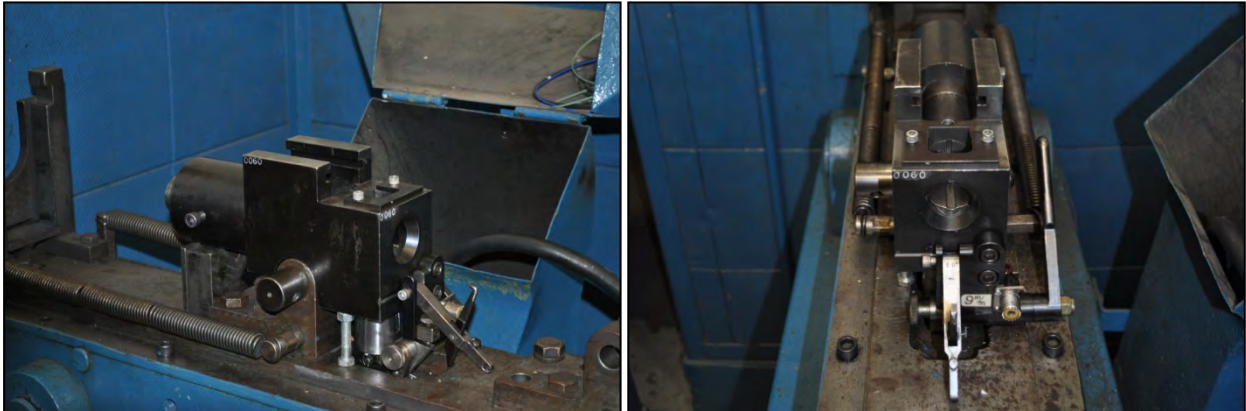
Figure. 6-B-3: Two views of the set-up for the 4.6mm, 5.7mm, and 9mm EPVAT Test
