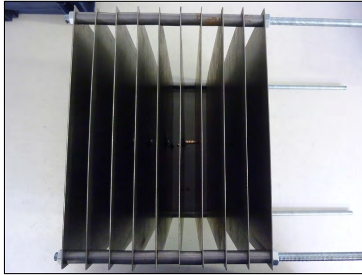
Figure. 6-B-12: A view of the multiple target array for the 4.6mm and 5.7mm Terminal Effects Test with ten (10) mounted and separated steel plates
